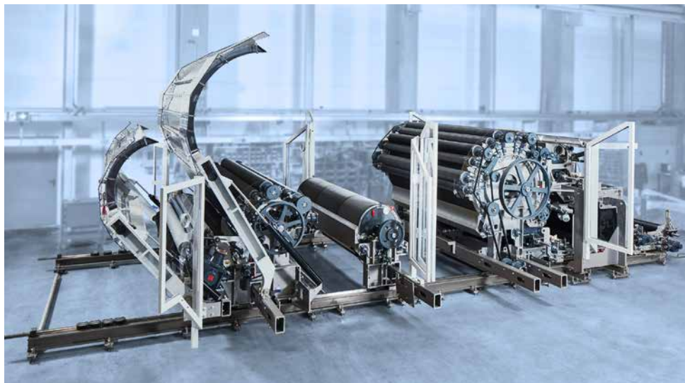
DiloSpinnbau MultiCard with special suction system
