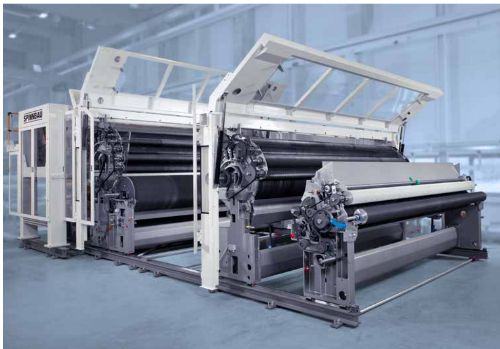
High-speed card, working width 5.1 m
