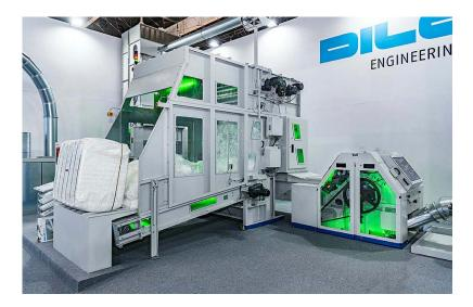
Another specialty is the fine opening stage installed over the material box of the new card feeder FRS-P where a high dosing accuracy is achieved in cross and longitudinal direction. A very even flock mat was a clear eye-catcher. Consequently, the high web quality at the VectorQuadroCard exit was a result of the high quality of synchronized fibre opening and web forming components which form a technological unit.
