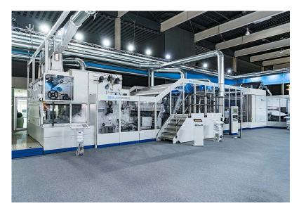
The revised HyperLayer NT for the presentation of the latest state-of-the-art highspeed precision layering technique showed new standards, which play an important role especially in hydroentanglement lines. In this application, it is important to achieve layering speeds up to 190 m/minute using sophisticated viscose fibres and a layering width of about 4 m while at the same time showing high layering precision in cross and longitudinal direction.
