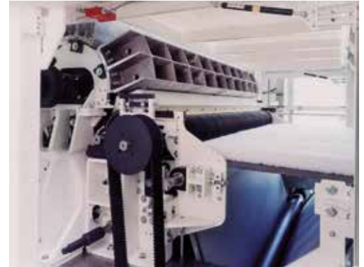
▲ Speiservliesmatte für aerodynamische Vliesbildner Web mat from the card feeder for aerodynamic web former
